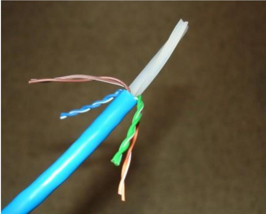
Now that the core has been removed, your next task is to straighten the wires that were previously twisted. The easiest way to do this is by using two pairs of tweezers. Use one set of tweezers to firmly hold the wire just beneath a bend, and the other pair to straighten the bend. The wires don't have to be perfectly straight, but the straighter they are, the easier your job will be.
