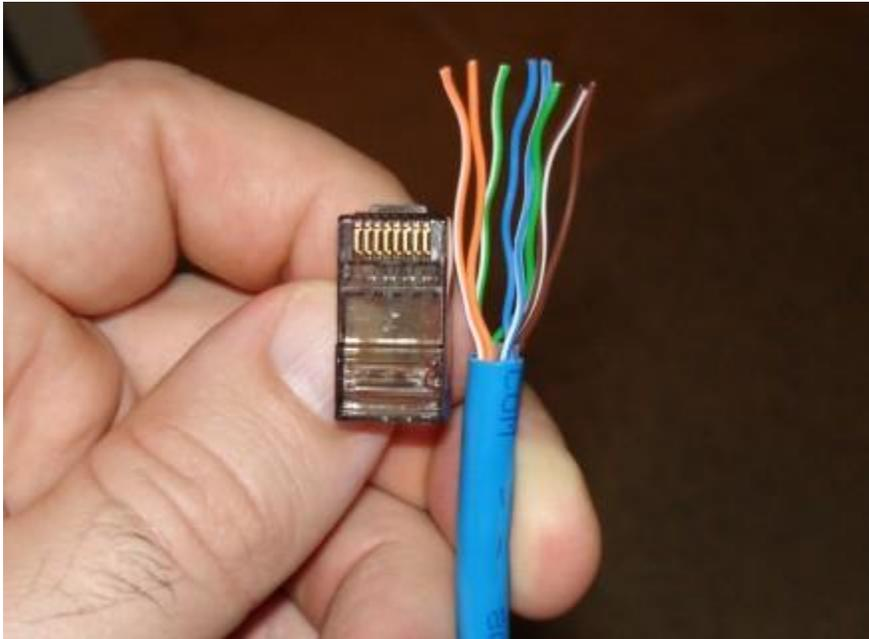
The easiest way to slide the RJ-45 connector onto the cable is to use your thumb to apply pressure to the cable in the spot where the wires are first exposed from beneath the insulation. This will help keep the wires in order.
