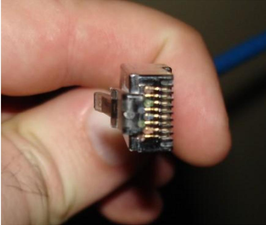
You should also verify that the wires are still in the correct order. It's easy for the wires to get out of order when installing the cable end. A quick check at this point will keep you from having to cut the cable end off and starting over later.
