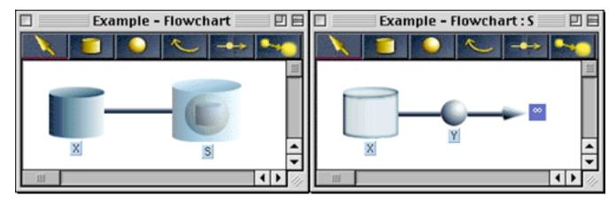
When you create the flow Y going from X, Berkeley Madonna creates a bundled flow or "pipe" in the top-level model connecting the original X icon and the submodel. This bundle reminds you that something in S is moving material in or out reservoir X. You could create additional flows in S connected to X and the appearance of the top-level flowchart would not change.
