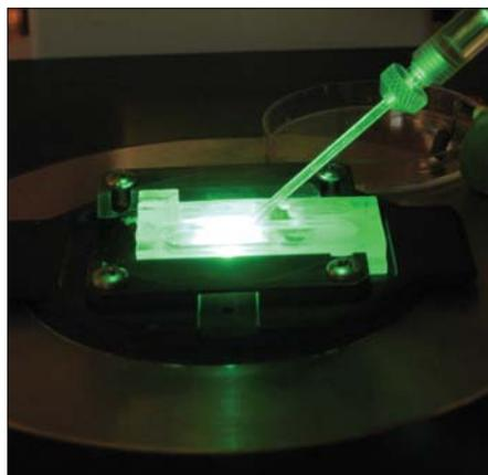
*Illuminating work: A glass electrode is used to measure the conductance of a membrane bearing light-switchable ion channels.*
